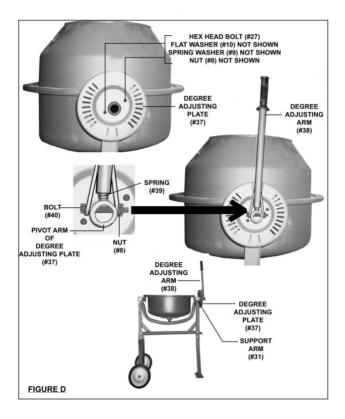
6. Secure the Degree Adjusting Arm (part #38) to the Pivot Shaft of the Degree Adjusting Plate (part #37), using one Bolt (part #40) and one Nut (part #8). (See Figure D.)
